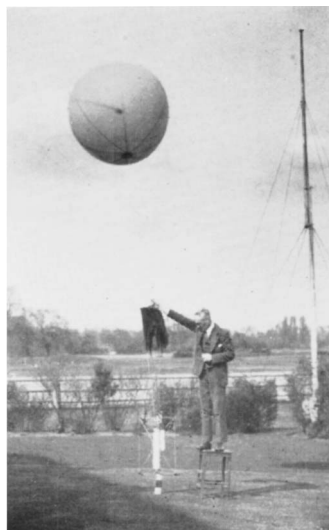
Mr. L. H. G. Dines launching a sounding balloon, with attached mechanism for air sampling, at Kew Observatory in 1936 (see ref. 26).
