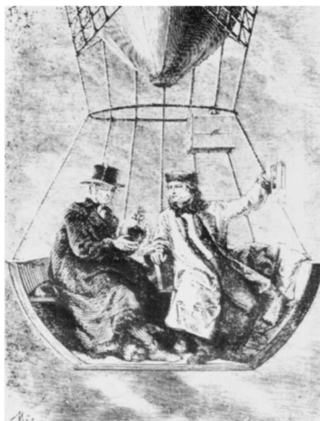
Gay-Lussac collecting air during a balloon flight in 1804, by turning the stopcock of an evacuated glass vessel. (The picture is included in J. Howard Appleton's "Beginners Handbook of Chemistry," Chauteauqua Press, New York, 1888; no reference to its origin is given.)
